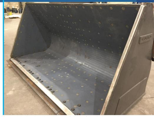
clay remained built up inside the bucket and the loading shovel bucket failed to fully discharge. The bucket required several hours of manual cleaning by plant engineers each day and also resulted in damaged equipment as the loading shovel operators tried to fully discharge the loads.
