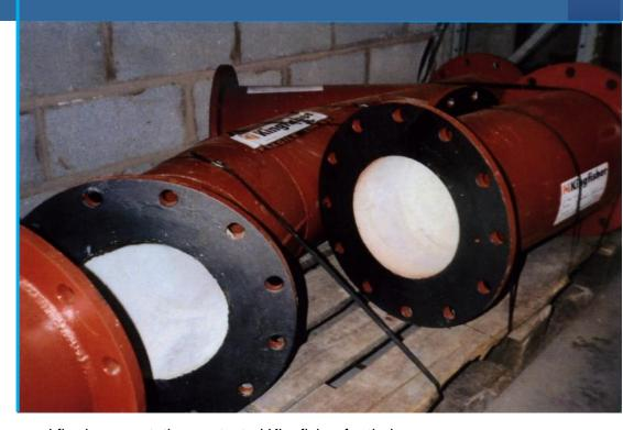
the coal and ash plant on a large coal fired power station contacted Kingfisher for their recommendations for use in handling hot clinker being charged via an ash reception hopper. Although the course clinker was suspended and conveyed hydraulically, the internal surface of the pipeline was subjected to severe abrasion and erosion.
