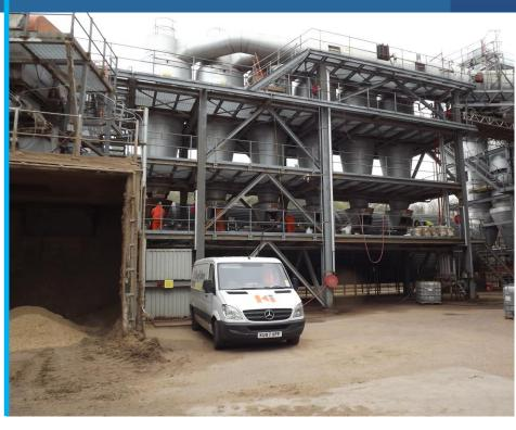
drying cyclones situated after the drying drum operating in a positive phase of conveyance. The structure albeit made from Hardox wear plate had suffered from extreme abrasion due to amount of contamination in the wood stream.
