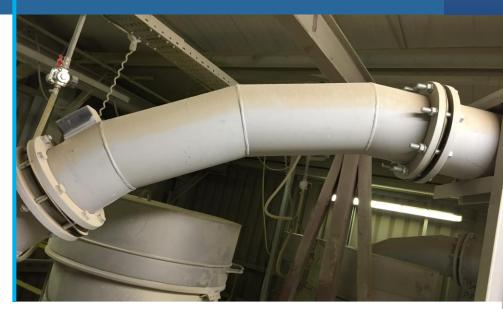
**Problem:** A major UK supplier of dry mortar experienced constant failures with their pneumatic pipe conveying systems and after constant attempts to sort the problem they eventually approached Kingfisher Industrial to find a solution as although an existing system was used, the pipes were still failing due to excessive wear which lead to product escaping to atmosphere resulting in plant shutdown to execute repairs and replacement.
