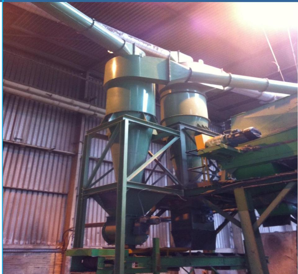
**Solution:** Having had success with our K-TEX polymer lining system within sand washing plants, we opted to line new steelwork with our 6mm thick material. All remanufacture, surface preparation, internal lining and painting of the equipment was carried in house as per the OEM's new design.
